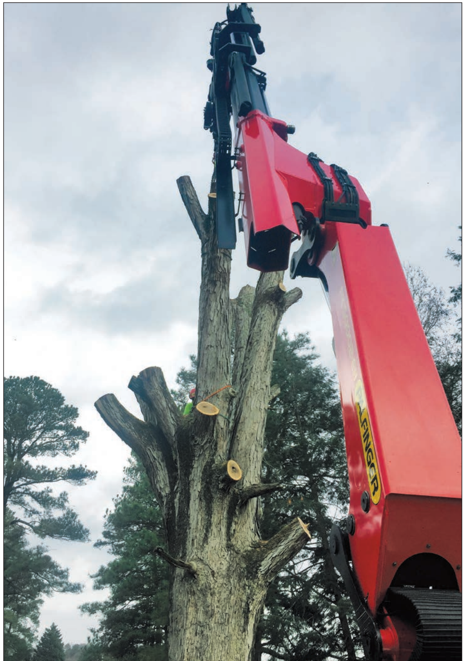
Photo 1: Day 1 involved limbing out the white oak with the grapple saw until we had manageable pieces to pick. Day 2, shown here, involved picking the trunk in manageable pieces and cleaning up. All photos courtesy of the author.
